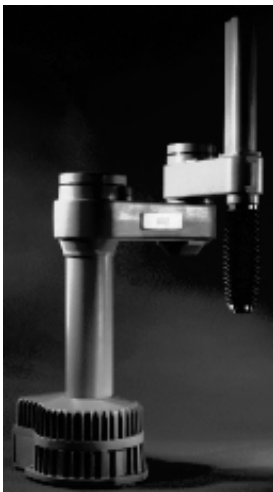
FIGURE 28.11 View of a SCARA robot (left) and cross-section through its direct drive arm transmission. (Courtesy of Adept.)
